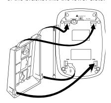
3. Plug one end of the supplied long modular cord into the TEL LINE jack on the back of the base.
